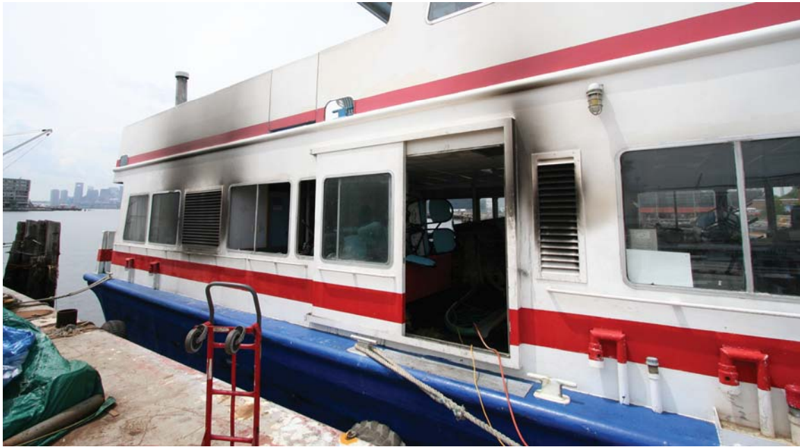
Figure 6. Smoke damage to outside of Massachusetts's main deck, starboard side.
